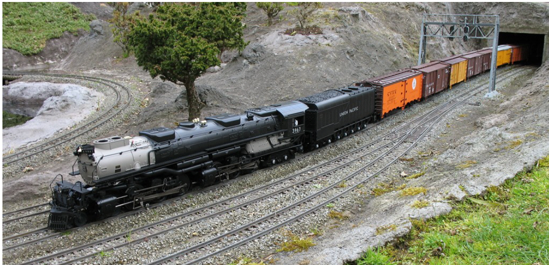
Bert Wettenschwiler's track using 145mm spacing on the straight and 155mm to 160mm on curves. Photo by Bert
